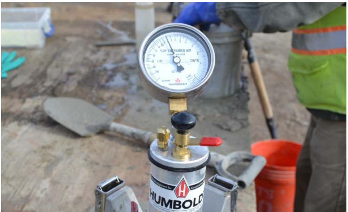
Filled and pressurized canister showing the percentage of air. Between 5 and 8% is required.
