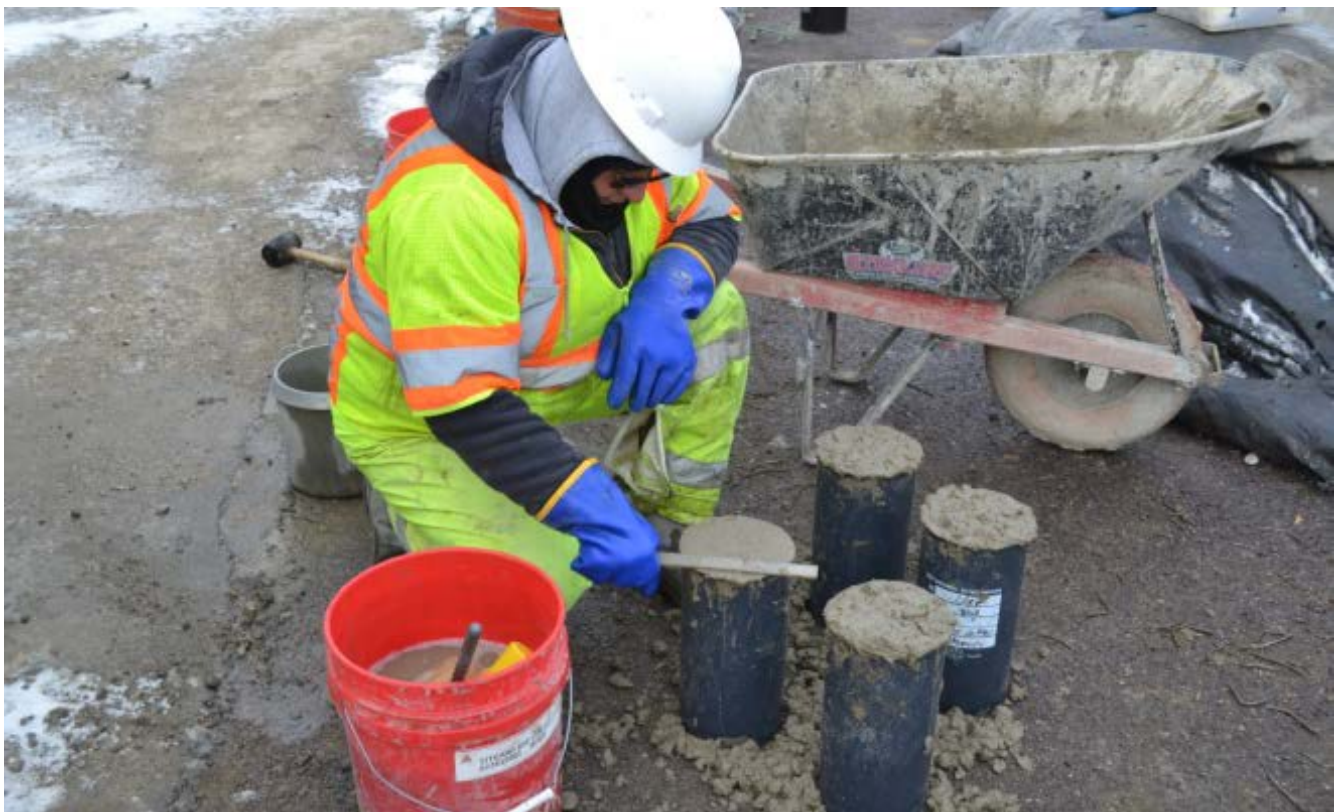
Filling the cylinders. Fill at one-thirds and 25 plunges to properly consolidate.
