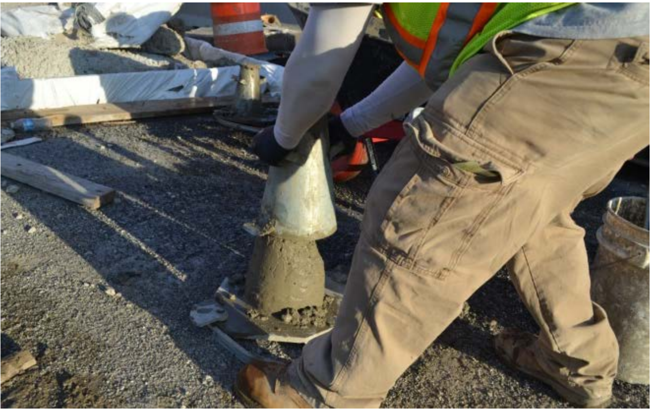
Cone being removed. Slump begins as soon as it is removed.
