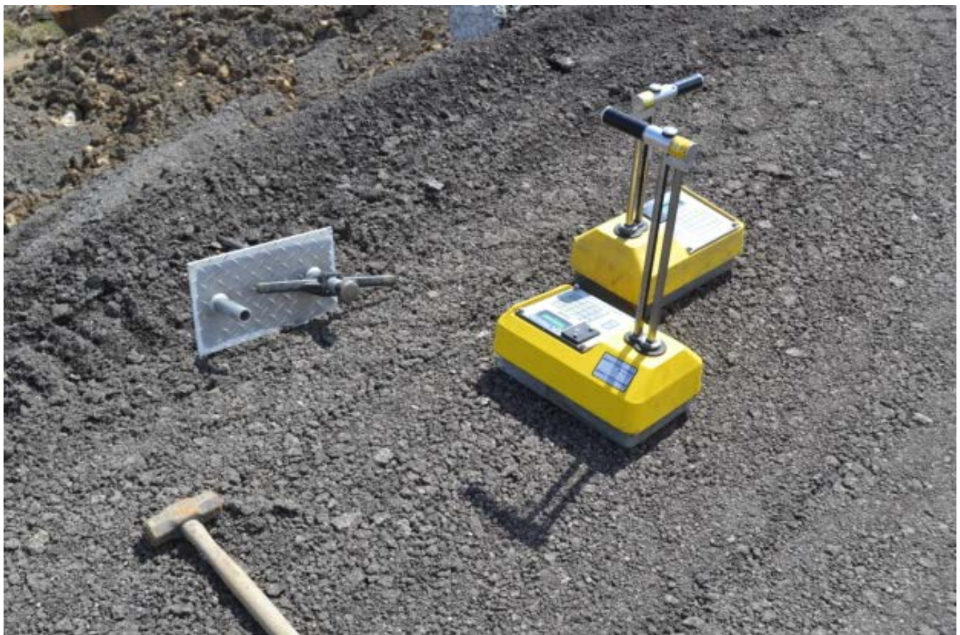
Nuclear density gauges and equipment for both the QC and QA Inspectors.
