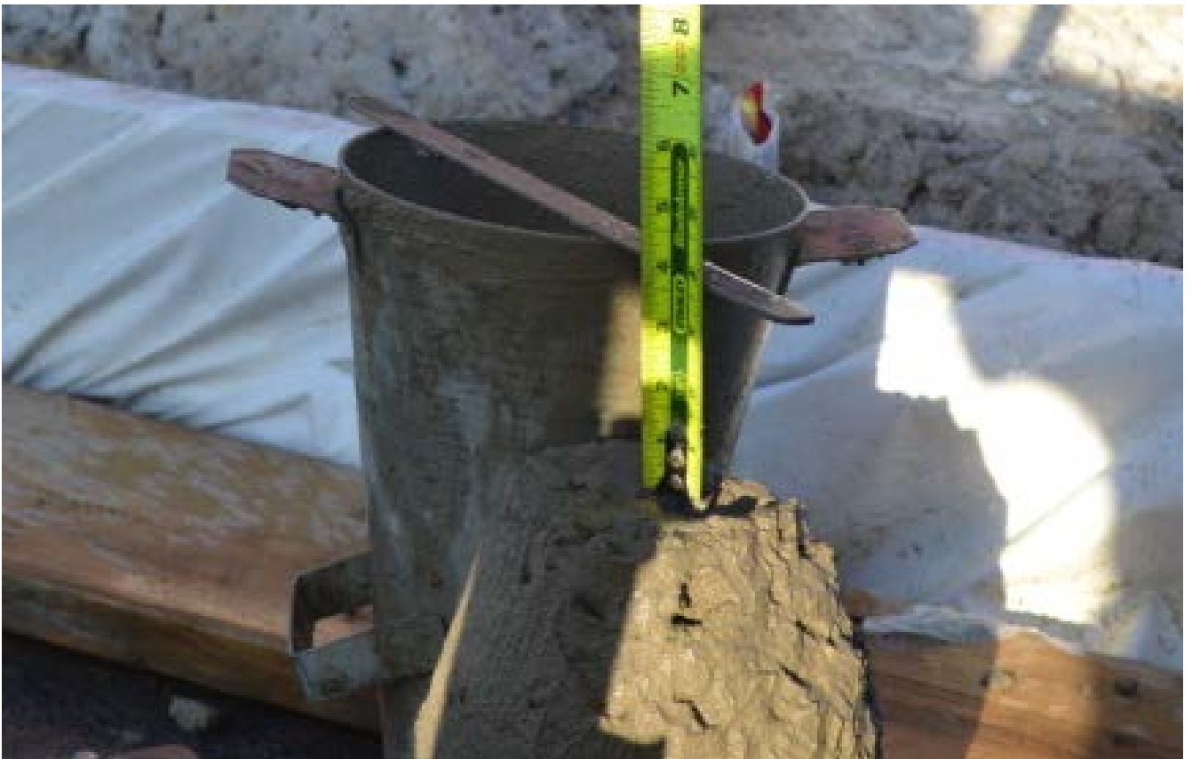
The slump is measured. The pump truck can pump concrete with 4" of slump.
