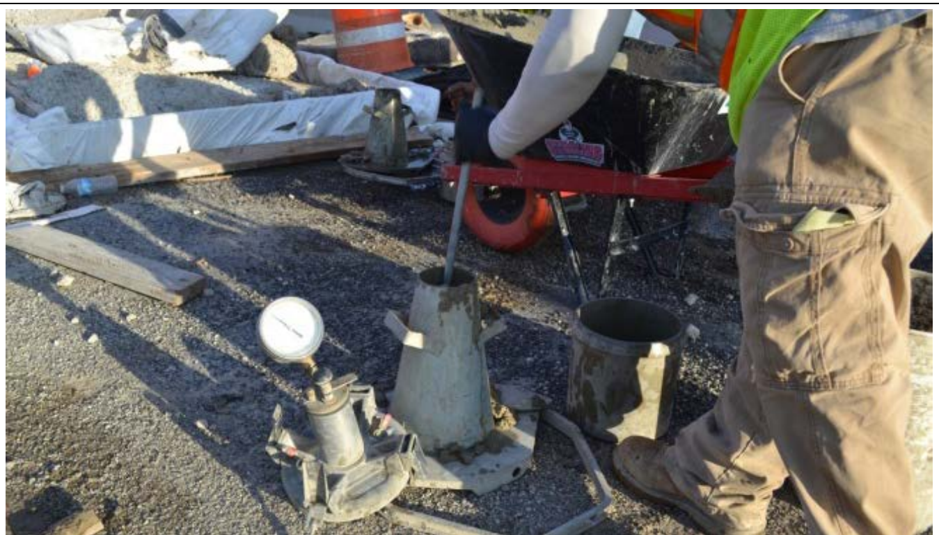
Loading the cone for slump. Fill at one-thirds and 25 plunges of the rod are required for proper consolidation.
