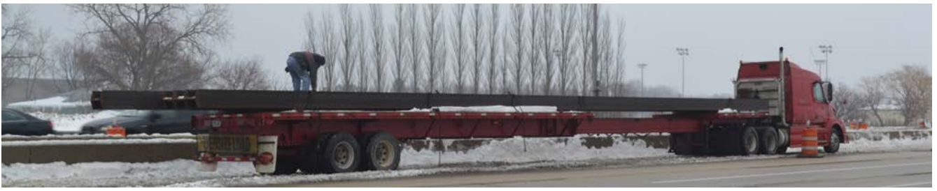
Semi-trailer delivering 85 foot H-piles. A special permit was required for this truck to travel on the highway.
