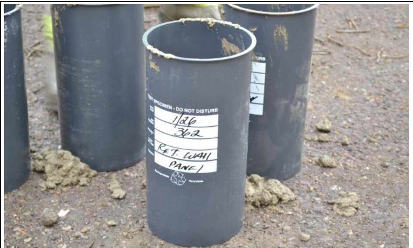
Cylinders properly marked for identification.
