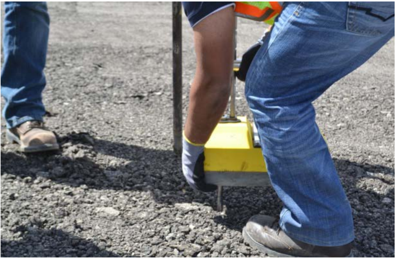
The QC Inspector properly setting the nuclear density gauge to test and obtain the reading.
