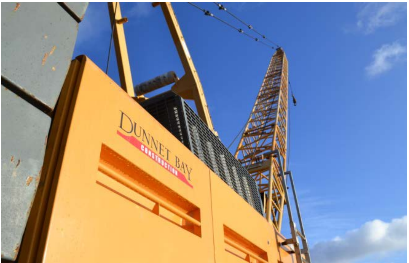
The contractor used a 300 ton crane with a 160 foot boom. All of this equipment was designed by engineers.
