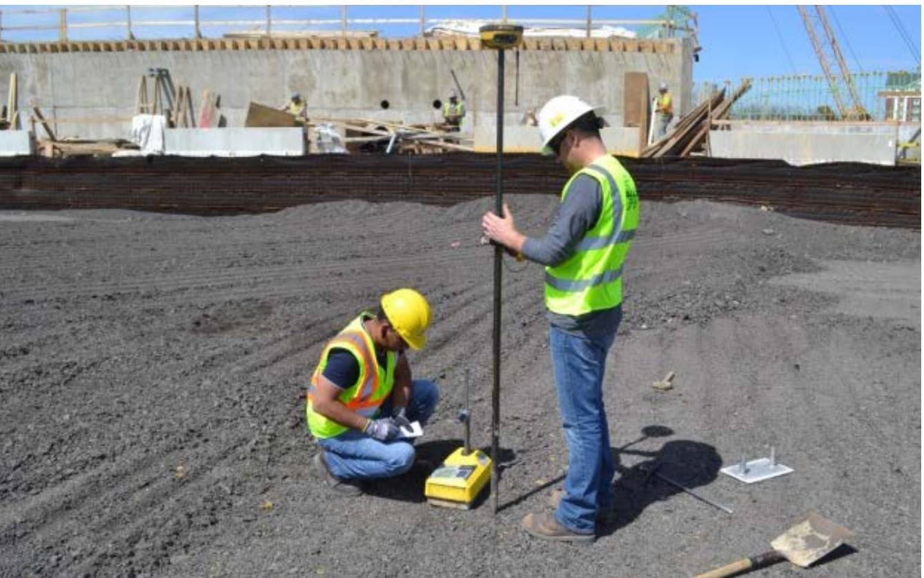
The QC Inspector, with a surveyor, locating both the horizontal and vertical position of a density reading.
