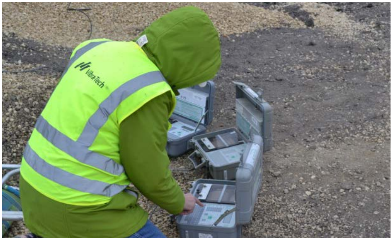
Engineer testing vibrations caused by driving piles near an existing high pressure gas main. If the vibrations became too great, the engineer would stop the pile driving.
