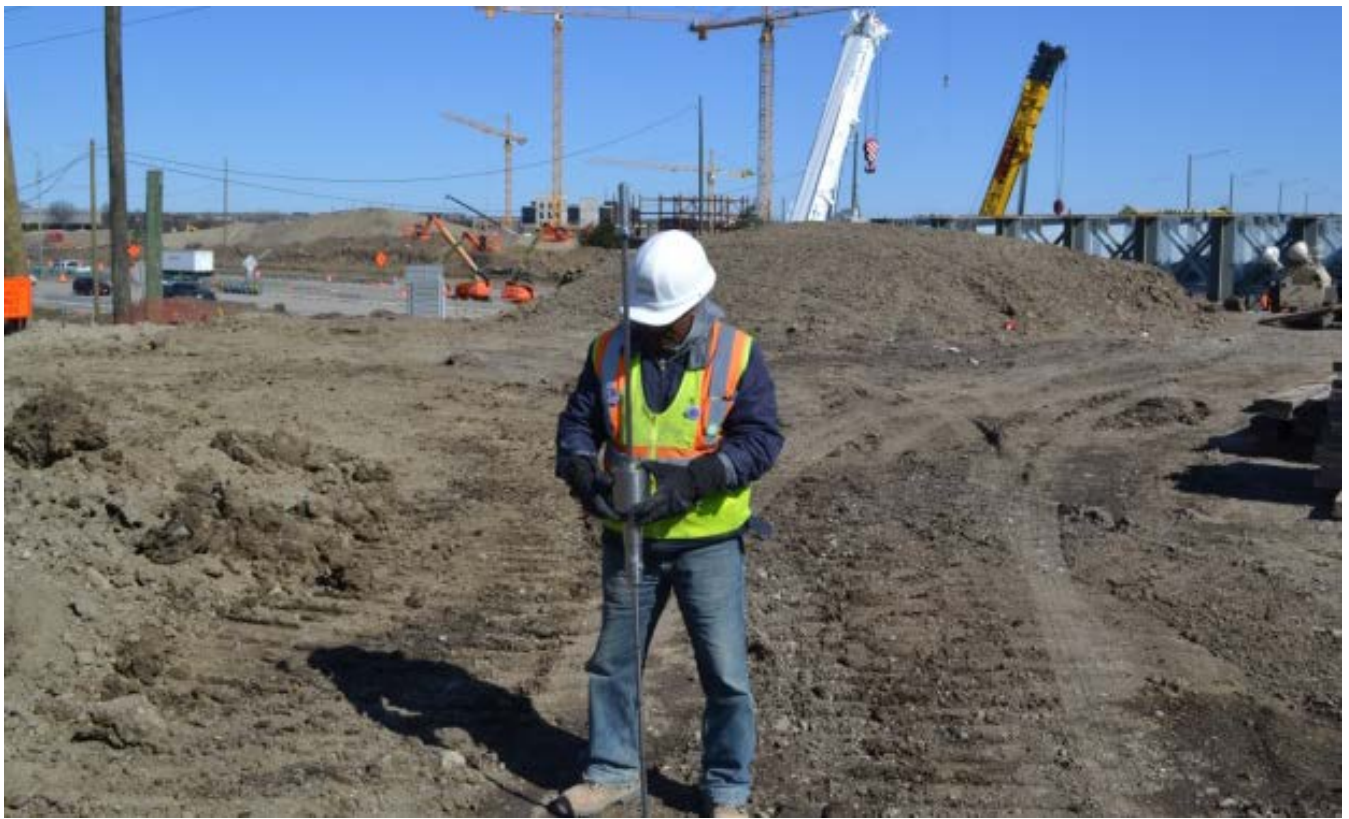
The QC Inspector using the DCP to test the subgrade after the topsoil was stripped and stockpiled.
