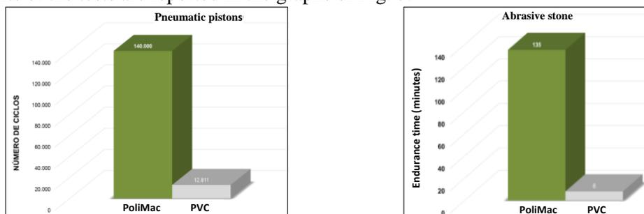
Figura 7. Results of the tests of the pneumatic piston and abrasive stone
