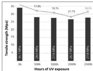
**Figure 4. Accelerated aging test - Tensile strength of the mesh.**
