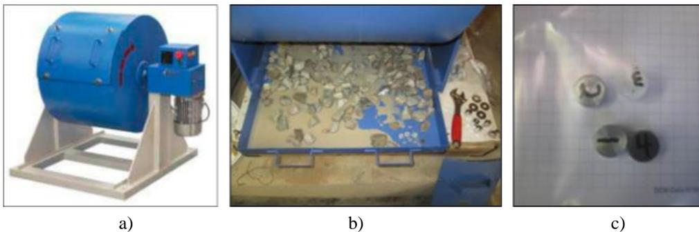
Figura 9. a) Los Angeles equipment, b) wear material used in the test and c) test bodies tested.
