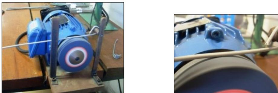
Figura 6. Abrasion test on abrasive stone
