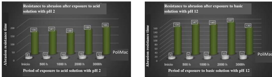
Figura 8. Difference of behavior of the samples submerged in extreme solutions with pH 2 and 12.
