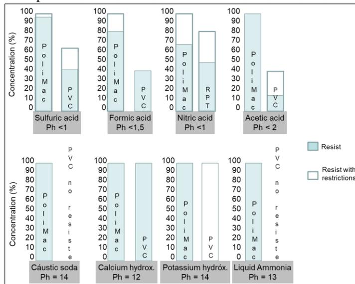
**Figure 3. Behavior of PVC and PoliMac exposed to different environments.**
