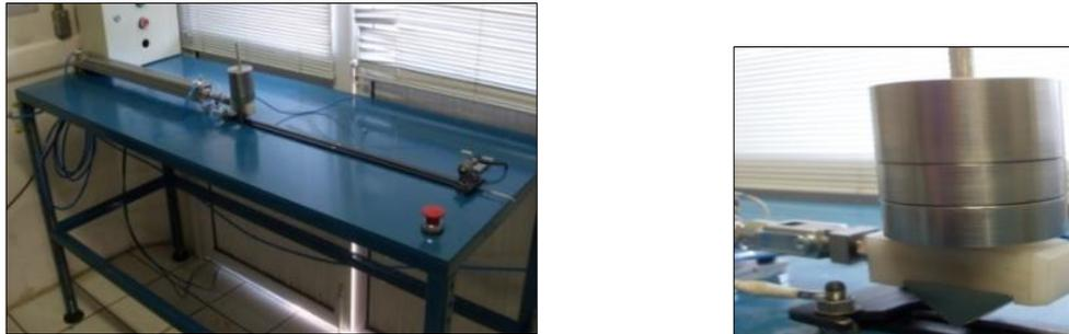
Figura 5. Abrasion test according to NBR 7577
