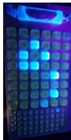
Figure 7: Tray under ultraviolet light lamp 24 hours later. FLUORESCENCE: POSITIVE FOR ENTEROCOCCUS
