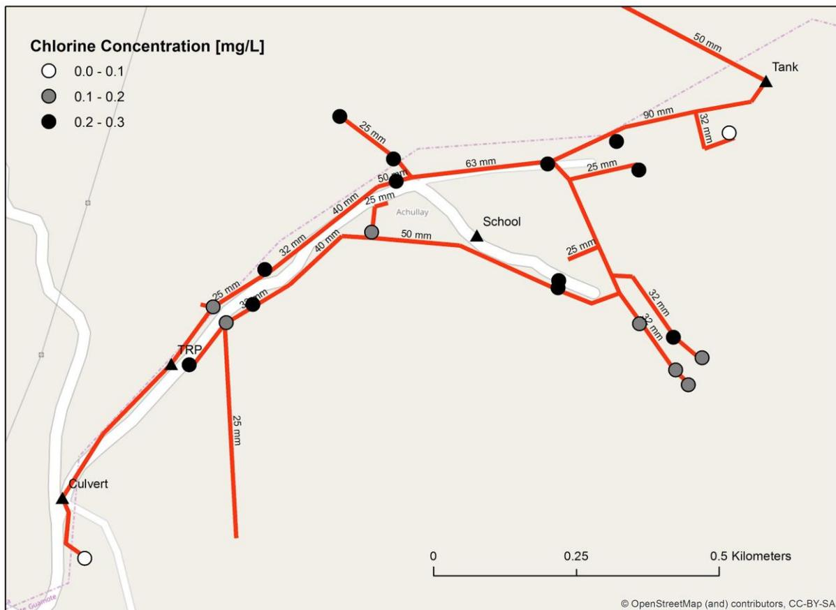
Figure 5. Free Chlorine Residual, Achullay, July 2018.
