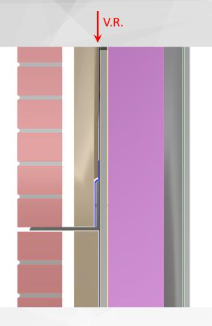
Location: Baltimore; cold year; **WUFI®** DC Met framing; (R-13+R-7.5ci) + vapor impermeable membrane - North 104 [Btu/h ft<sup>2</sup>] £ >400 68 Temperature 300 200 32 10/1/2018 100 0 -4 100 [in/h] >10 80 . Rel. Humidity [%] 60 1 Water Conte 0.1 40 6.24 20 0.01 0.001 0 0 3.5 2 0.041 0.491 3.63 0.492 1 \*Red Matt Clay Brick \*Air Layer 25 mm \*Gypsum Board \*Gypsum Board \*Roxul CavityRock \*Low Density Glass Fibre Batt Insulation \*Perm-A-Barrier Wall Membrane Cross Section [in]
