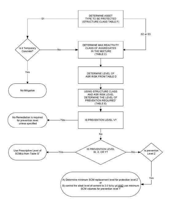
Note 1: The prevention level may be reduced by one level if low alkali cement ( $\leq 0.70$ ) is used.
