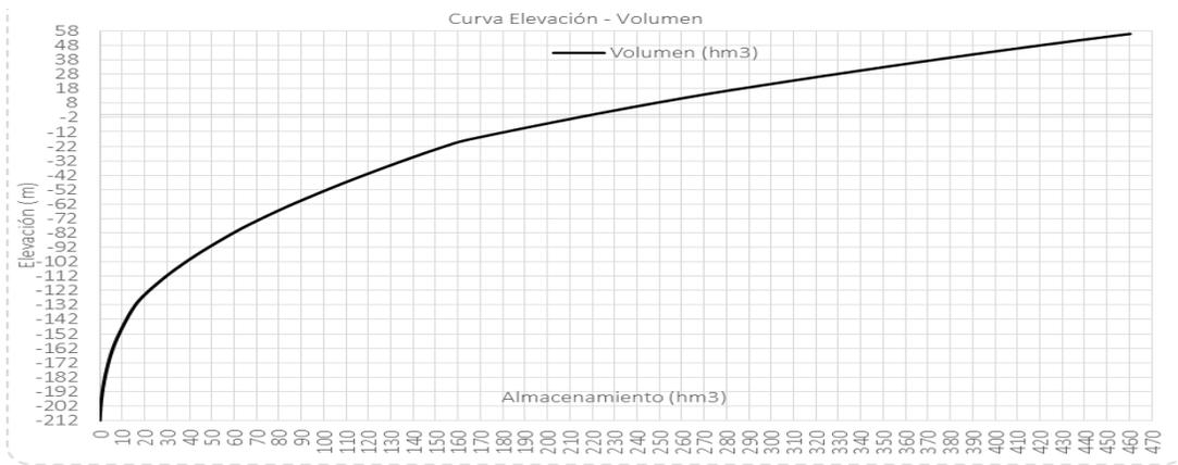
**Figure 4. Elevation curve - Volume. Typical storage areas.**
