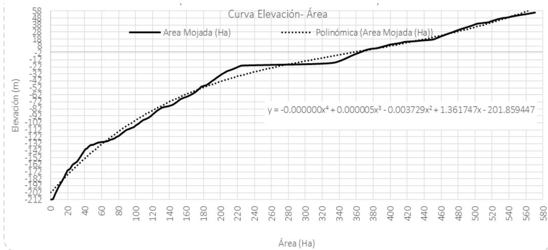
**Figure 3. Elevation-Area Curve. Typical storage areas.**
