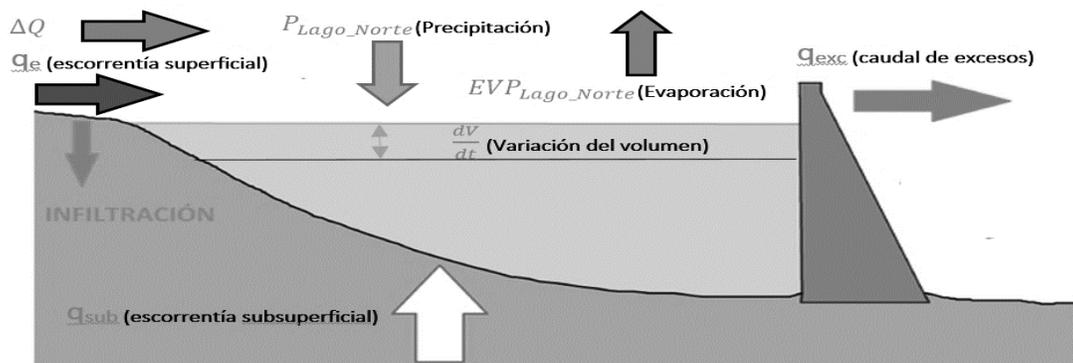
**Figure 2. General outline of the hydrological balance in the pit. Filling analysis on a daily basis.**
