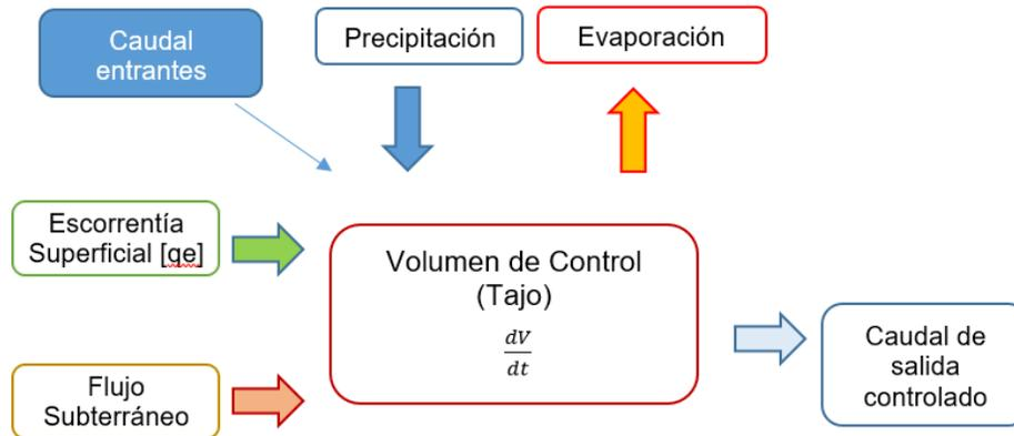
**Figure 1. Flow diagram of the variables of the water balance in a control volume.**
