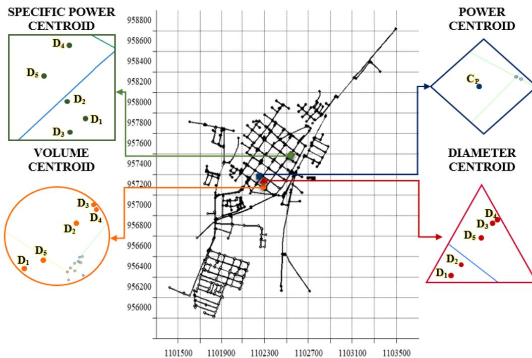
**Figure 3. Localization of Centroids in the Bugalagrande network. ● Volume Centroid; ■ Specific Power Centroid; ◆ Power Centroid; ▲ Diameter Centroid.**
