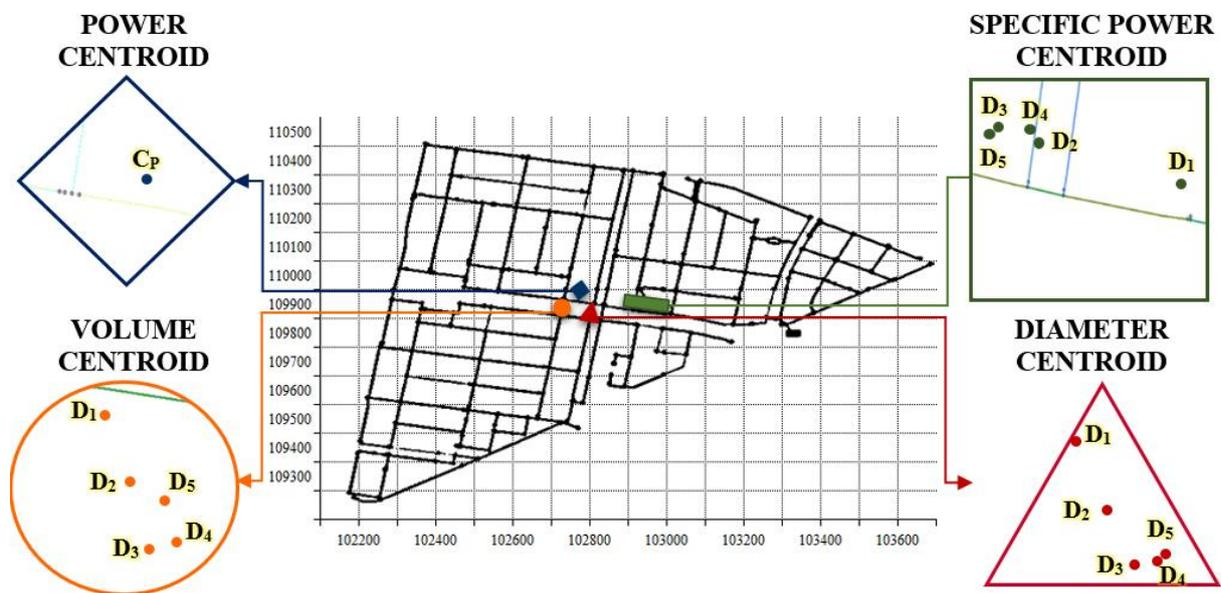
**Figure 6. Localization of Centroids in the Subsector 4 network. ● Volume Centroid; ■ Specific Power Centroid; ◆ Power Centroid; ▲ Diameter Centroid.**
