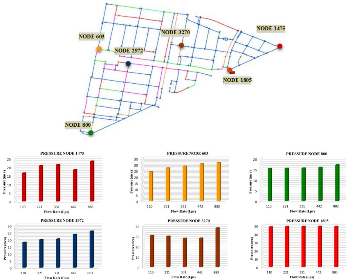
**Figure 4. Pressure on nodes of the Subsector 4 network.**
