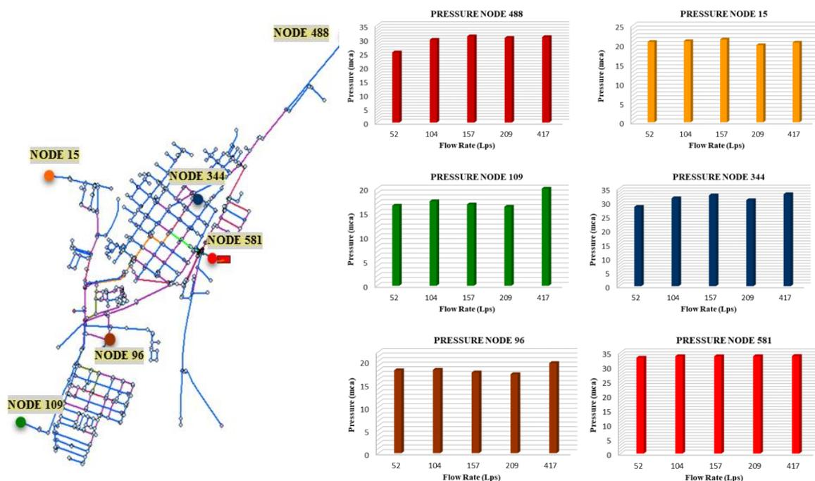
**Figure 2. Pressure on nodes of the Bugalagrande network.**
